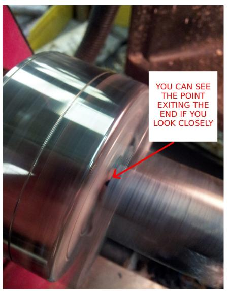
If drilling completely though a blank, you may be able to watch where the blank ends in the gap of the spinning jaws for exiting which can help in knowing when to stop advancing.
