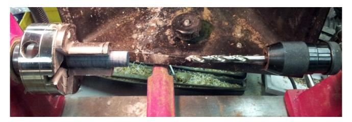
In addition, a chuck to hold the drill bits in the tailstock. This chuck must not rotate, so avoid purchasing a drill chuck denoted as "live". A 1/2" drill chuck is recommended in order to accommodate most common drill bit sizes.
