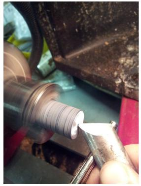
piece. You'll be able to see the center point of rotation. Use the skew chisel point to dig in a small hole exactly at that center. This will ensure that the drill point is placed exactly where it is needed.
